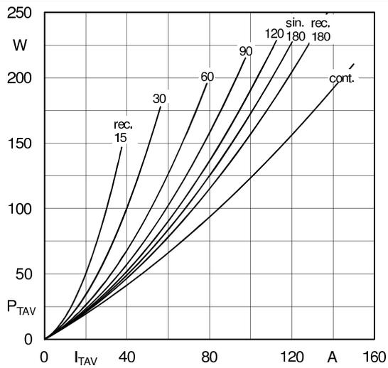
Fig. 1L: Power dissipation per thyristor/diode vs. on-state current
