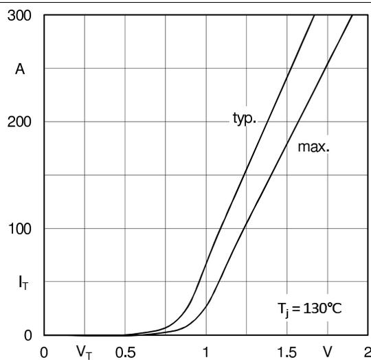
Fig. 7: On-state characteristics
